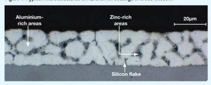
Figure 1a: ZINCALUME® steel AZ150 (superseded)
