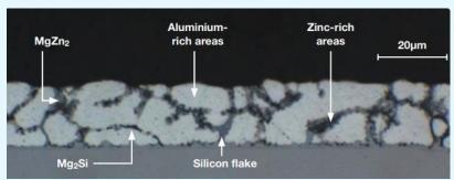
Figure 1b: Next generation ZINCALUME® steel AM125
